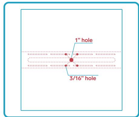
1. Trace the slots of the support bracket to the top surface of the ceiling tile.
