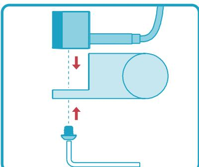
3. Insert the BRIO and USB-C cable into the camera mount, and mounting the screw with  $5/32"$  hex key.
