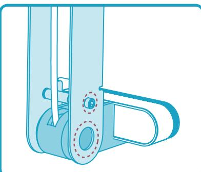
4. Re-install camera mount and tighten screw with  $5/32"$  hex key.
