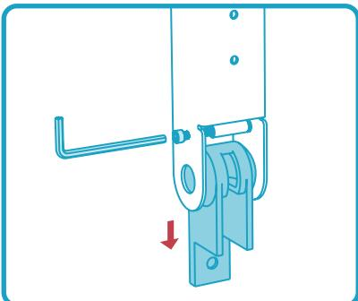
1. Loosen screw and remove the camera mount.
