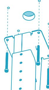
1. Feed the four screws through the pre-drilled holes.
