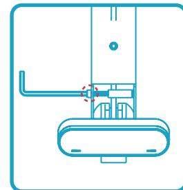
1. Loosen the screw to adjust the camera angle.
