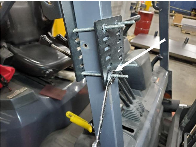
Determine mounting height on post. Add backing plate and hardware.
