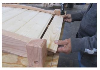
12. Put the other end floor board. Fasten the floor boards with small screws.
