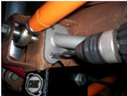
Drill two 3/8" holes in the driver's side control arm mount using the axle brace flange as a guide. Install the 2 supplied 3/8" bolts and locknuts into these holes.
