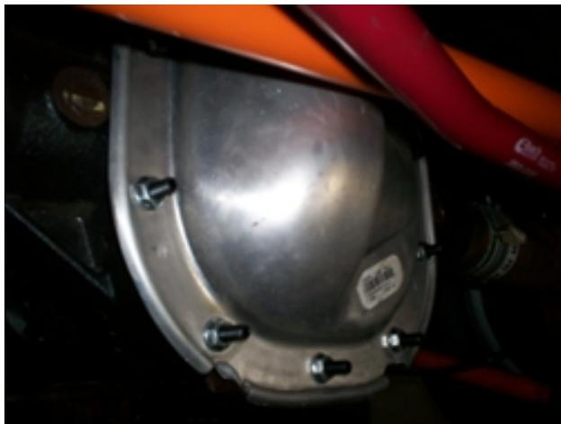
**Important!!** Only remove and install one cover bolt at a time to prevent oil leaks.
