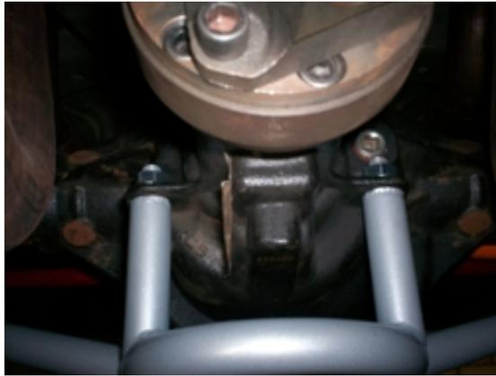
Final torque the 1/2" cover plate bolts and the front axle brace stud nuts to 50 lb-ft.
