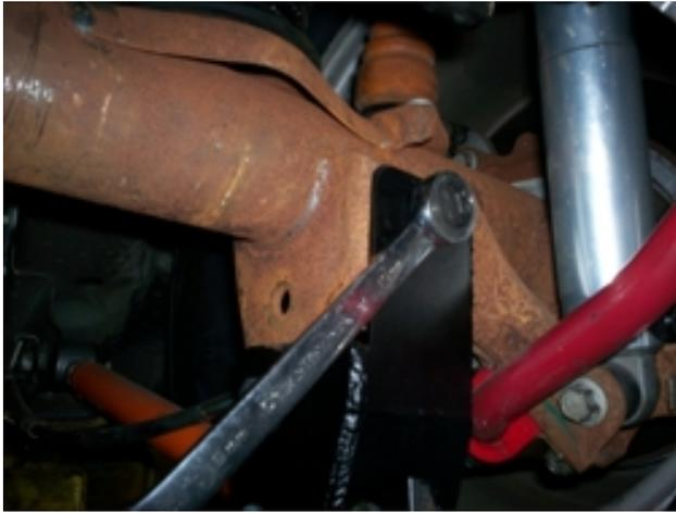
**Important:** If installing CHE Lower Control Arm Anti-Squat Brackets or brackets from another manufacturer, they should be installed prior to proceeding with installation of axle brace. Please print a copy of our supplemental installation instructions for Bolt-On Relocation brackets from other manufacturers from the Installation/Tech section of our website for detailed instructions. The CHE Brackets will not require the supplemental installation instructions.
