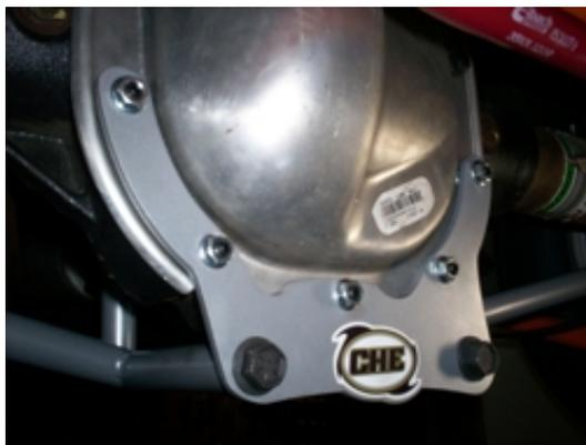
Install the cover plate over the cover plate studs and nuts on the differential housing. Install the supplied flange nuts on the studs. Torque the nuts to 25 lb-ft.
