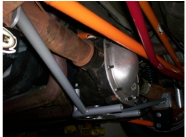
**NOTE:** In certain cases, the holes in the axle housing flanges (near the pinion flange) are not present. In this case, the holes must be drilled following the instructions included with the axle brace before installation can continue.
