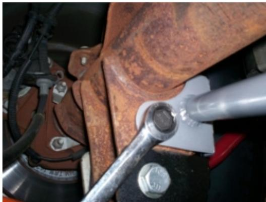
Install the supplied 12mm flange bolts into the weld-nuts on the control arm mounts on both sides of the axle. Do not fully tighten these bolts at this time; the bolts should be loose enough to still allow slight final positioning of the axle brace.
