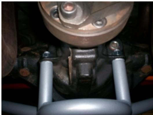
Install the supplied nuts onto the Axle Brace studs on the front of the axle housing. Do not fully tighten the nuts at this time; they should only be tight enough to still allow slight final positioning of the axle brace.
