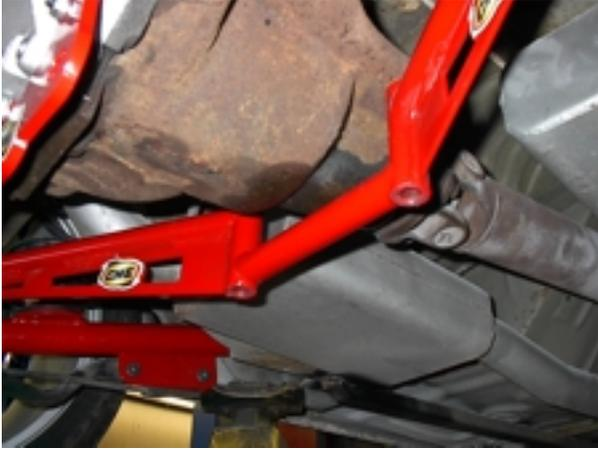
Remove the 2 Front Differential Center Section bolts from the Axle Brace using a  $\frac{3}{4}$ " wrench or socket.
