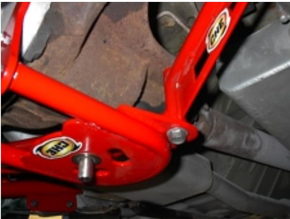
Install the Tie-In Loop, re-using the 2 bolts removed in step 6.
