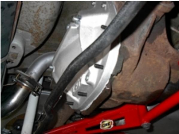
Install the 5 supplied cover studs into the lower 5 holes of the differential cover using a 5/32" Allen wrench.
