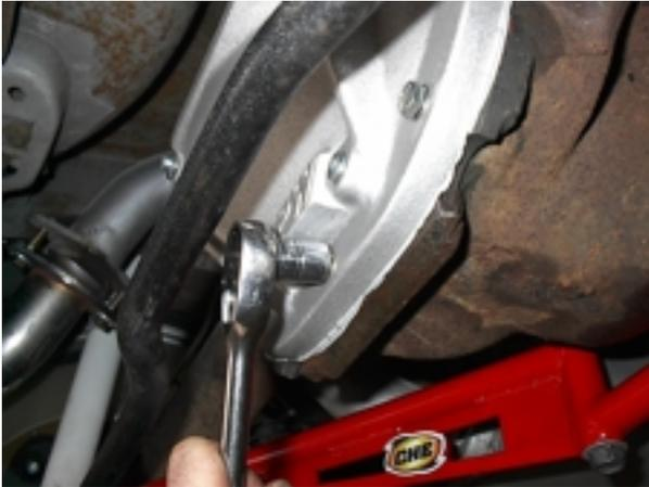
Remove the lower 5 bolts from the differential girdle.
