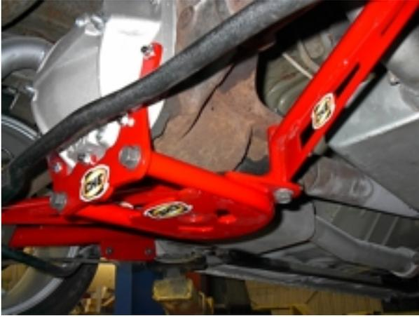
Torque the 2 Front Differential Center Section Axle Brace bolts to 50-60 lb-ft.
