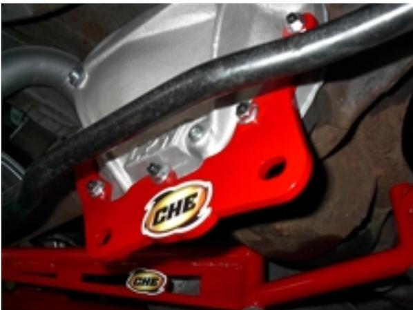
**IMPORTANT:** The cover plate must sit flush to the flange of the differential girdle. Due to variations in castings, it may be necessary to trim either the differential girdle or the differential plate to allow a flush fit.
