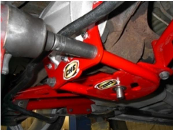
Install the supplied Cover Flange Bolts into the loop using a  $\frac{3}{4}$ " wrench or socket. Torque the bolts to 50-60 lb-ft.
