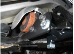
Using the installation instructions included with the K-member brace, install the brace on the vehicle. **Do not fully tighten the bolts at this time.**
