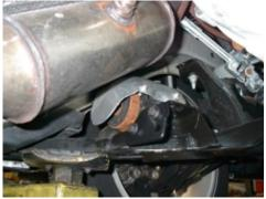
Using the supplied flange bolts and nuts, install the adapter plates onto the K-member flanges. If needed, enlarge the drilled holes with a round file or other suitable tool. **Do not fully tighten** the bolts at this time.
