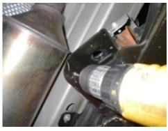
A. Using a center punch, mark the k-member flanges at the designated locations on the template. Because you will be drilling at an angle, it is very important that these punch marks be accurate and as deep as possible.
