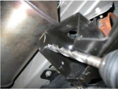
Using a good sharp drill bit, enlarge the holes to 7/16"
