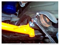
C. Install the 10mm bolts (17mm Bolt Head) and flat washer into the rear mounting holes of the brace, but *do not tighten them at this time*. There should be enough slack in the brace to allow final positioning of the brace. Do this on both sides of the brace.
