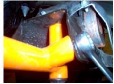
A. Snug up the rear flange bolts until they are just tight enough to take any slack out of the bolt. Do not final torque it at this time. This step will insure proper alignment of the brace without causing deformation of the k-member flange.
