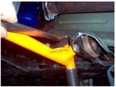
B. Torque both of the control arm mount bolts to 100 ft-lbs (135N-m).
