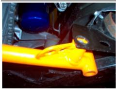
A. If present, remove the factory K-member brace from the vehicle by removing the 4 fasteners that retain it to the K-member. Note that not all vehicles have a brace from the factory. 2011-Current vehicles require modification described in step 1a.
