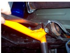
C. Place a washer over the provided 14mm bolt and install it through the tubular standoffs of the brace and into the front control arm bushing mount holes, re-using the factory locknut. *Do not fully tighten them at this time*. There should be enough slack in the brace to allow final positioning of the brace. Do this on both sides of the brace.
