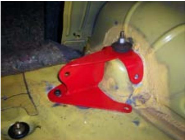
5a. Place the shock tower brace ends over the shock studs. Note that the Driver's side is marked with a "D" and the Passenger's side is marked with a "P" cut into the baseplate.
