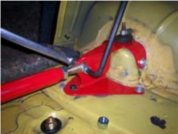
Adjust the length of the bar. The bar should be lengthened until it is applying light outward pressure to the brace ends.
