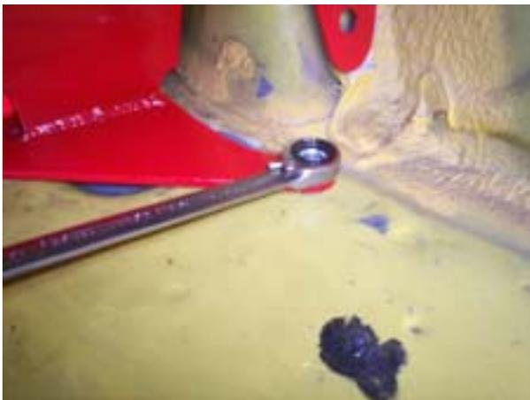
6b. Install the supplied 3/8 Self-Tapping Flange Bolts in the drilled mounting holes. Torque the fasteners to 25 ft-lbs. ***Do not over-tighten the fasteners.***
