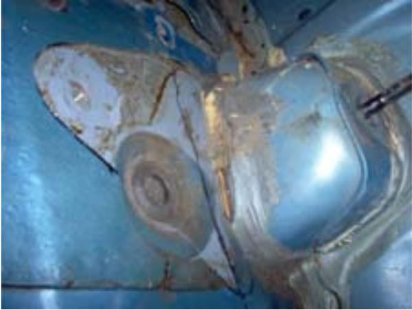
Using a suitable tool, cut away and remove the sound deadener from under the flange.
