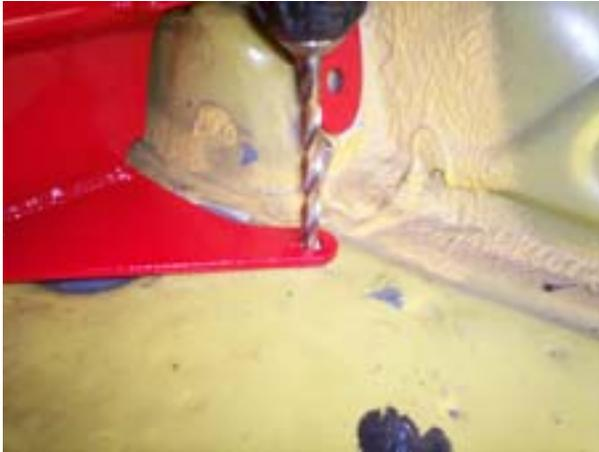
6a. ***Before drilling, inspect the area under the mounting holes to insure that there are no objects under the vehicle that may be damaged during drilling.***
