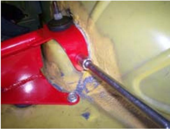
7b. Install the supplied 3/8 Self-Tapping Flange Bolts in the drilled mounting holes. Torque the fasteners to 25 ft-lbs. **Do not over-tighten the fasteners.**
