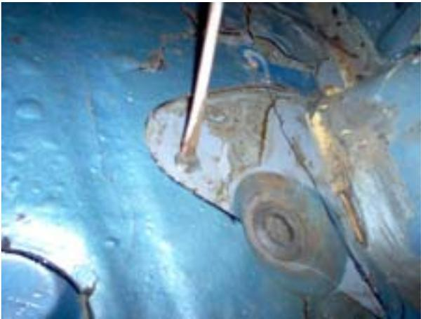
Remove the body sealer plugging a weld-nut that is located on the framerail of the vehicle using a suitable tool. This weld-nut should be located under the inboard holes of the Shock Tower Brace.
