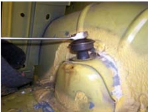
With the vehicle on the ground, remove the retaining nuts and bushings from the tops of the shocks.
