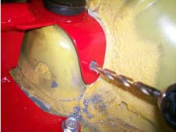
7a. **Before drilling, inspect the area behind the mounting holes to insure that there are no objects under the vehicle that may be damaged during drilling.**
