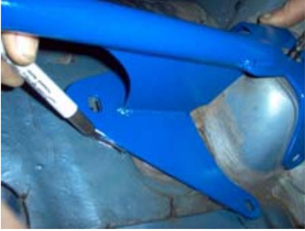
Place the brace over the shock studs and trace the lower flange onto the sound deadener.
