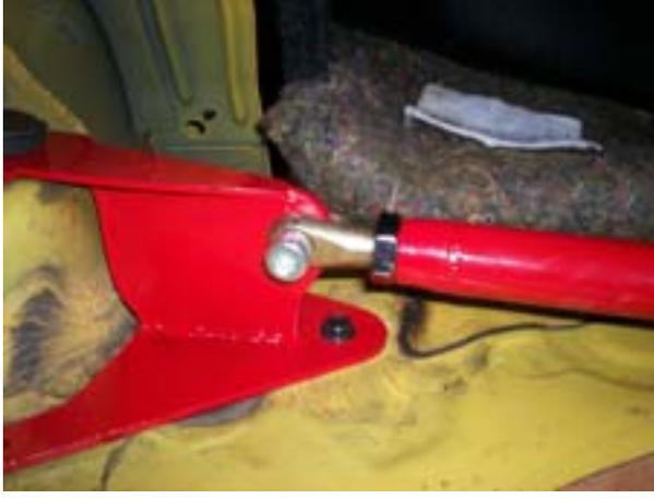
5b. Install the clevises in the bar. Note that the left hand threads are marked with a groove on both the bar and the clevis jam nut. The clevises should be fully threaded into the bar.
