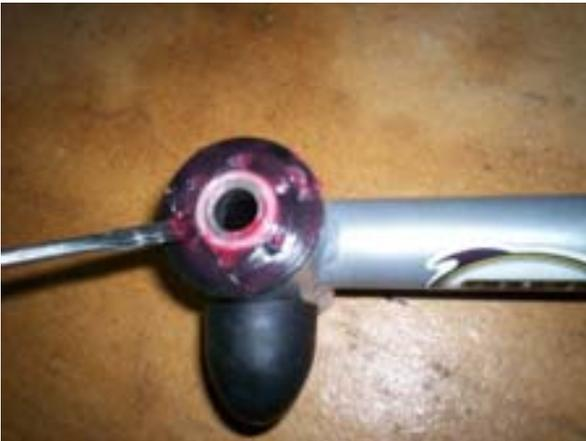
If installing a new Upper Control Arm: Using the provided assembly lube and brush, coat the bushing faces and the face of the control arm mount where the bushings make contact.
