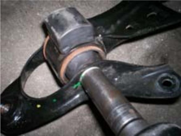
Using a 21mm & 18mm socket, remove the stock control arm from the mount. Save the bolt and nut for re-use.
