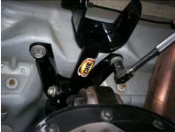
Coat the 2 rear Control Arm Mount retaining bolts with the Supplied Threadlocker compound.
