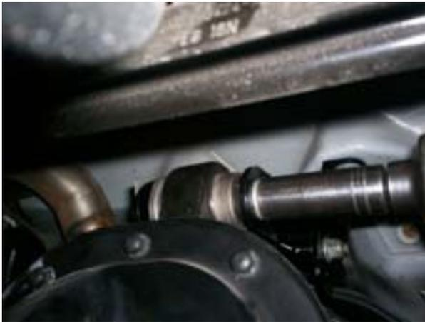
Install the factory flag-bolt and nut on the rear (axle housing side) of the upper control arm. If the rear axle has shifted during installation, it may be necessary to use a floor jack under the pinion side of the differential to align the bolt holes.
