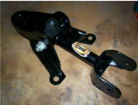
Using the factory nut and bolt, install the control arm onto the Upper Control Arm Mount, making sure that the pinion snubber is in the proper position. Torque the bolt to 100lb-ft. Use either of the 2 sets of mounting holes depending on your desired application.
