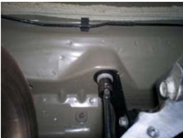
Using an 18mm socket, remove the 2 bolts retaining the Upper Control Arm Mount to the body of the vehicle. Save the bolts for re-use.
