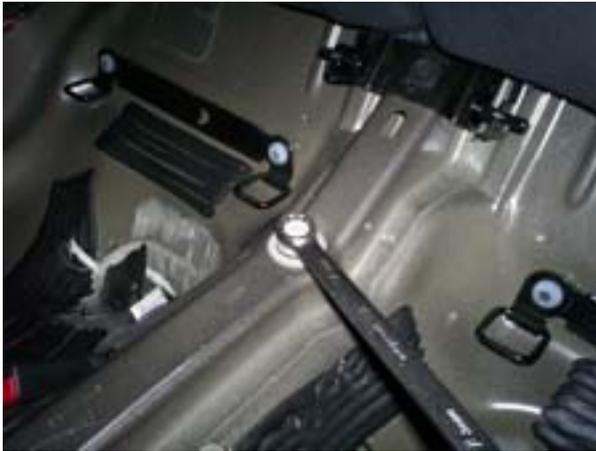
From the inside of the vehicle, remove the stock Upper Control Arm Mount front bolt using an 18mm wrench or socket. Save the bolt for re-use.
