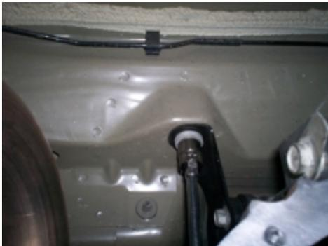
Remove the 2 bolts retaining the Upper Control Arm Mount to the body of the vehicle. Save the bolts for re-use.
