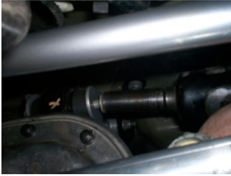
Install the factory flag-bolt and nut on the rear (axle housing side) of the upper control arm. If the rear axle has shifted during installation, it may be necessary to use a floor jack under the pinion side of the differential to align the bolt holes.
