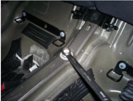
From inside the vehicle, install the factory Upper Control Arm Mount front bolt using an 18mm socket. Torque the bolt to 175N-m (129lb-ft). Install the rear lower seat cushion at this time.
