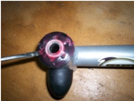
Using the provided assembly lube and brush, coat the bushing faces and the face of the control arm mount where the bushings make contact.
