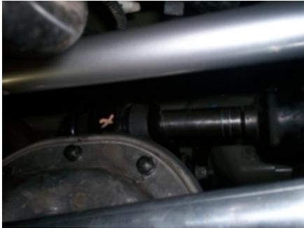
Remove the Control Arm Bolt from the Axle Housing and remove the Control Arm and Mount from the vehicle. Save the flag-bolt and nut for re-use.
