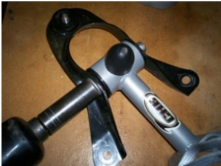
Using the factory nut and bolt, install the new CHE control arm onto the Upper Control Arm Mount, making sure that the pinion snubber is in the proper position. Torque the bolt to 175N-m (129lb-ft).
