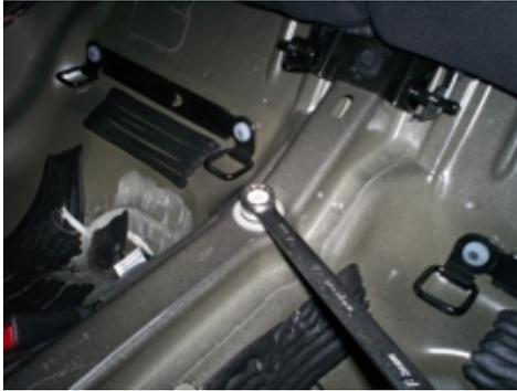
From the inside of the vehicle, remove the Upper Control Arm Mount front bolt using an 18mm wrench or socket. Save the bolt for re-use.
