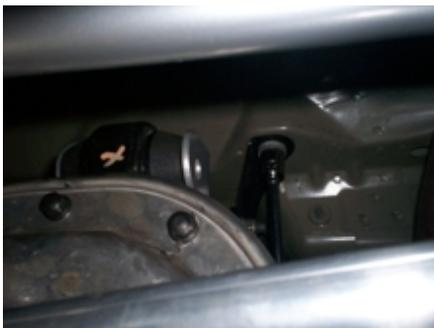
Install the Upper Control Arm assembly in the vehicle. Install the 2 rear Control Arm Mount bolts. Torque the bolts to 115N-m (85lb-ft).
