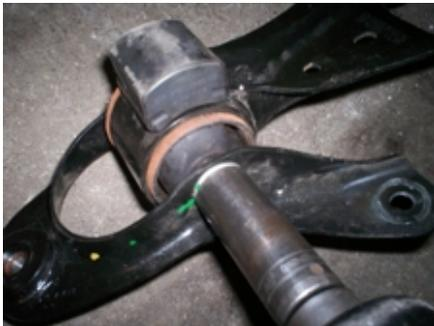
Remove the stock control arm from the mount. Save the bolt and nut for re-use.
