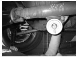
The pinion gear angle can be measured from any surface that is either exactly parallel or exactly perpendicular to the pinion, such as the pinion flange or a bearing cap.
