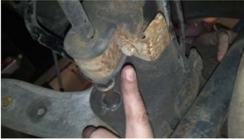
The sway bar bushings and bracket on the axle interfere with the removal of the axle side lower control arm bolt. *It is not necessary to remove the swaybar completely.* Remove the bolts for the bushing bracket on the axle housing and slide the bracket and bushing over to make room. Save the hardware for re-use.
