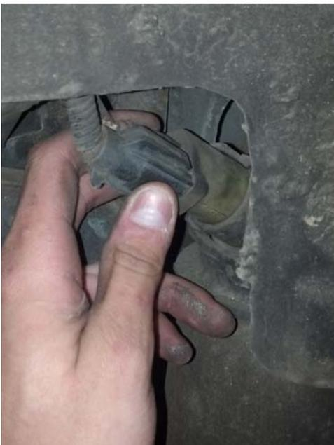
Release any air pressure on the air spring by rotating the air bag solenoid on the top side of the air spring counter-clockwise and pulling outward on it. **Be prepared for air to escape from the spring as it may rush out quickly.** Leave the solenoid loose until the new control arms have been installed.
