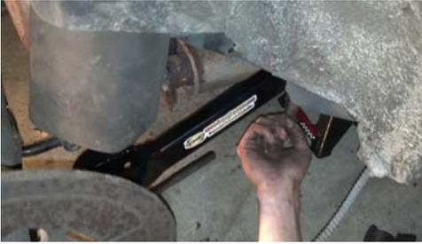
Install the new control arm following the reverse procedure of removal (forward mounting bolt first), using the new hardware provided with the control arms. Do not fully tighten the bolts at this time.
