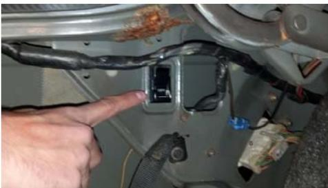
Located in the trunk on the driver's side, there is a switch to shut off the air ride. It is to the left of the trunk hinge. It may be behind some of the carpeted panels, so be sure to look carefully.
