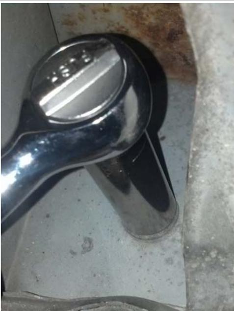
**ONLY REMOVE ONE CONTROL ARM FROM THE VEHICLE AT A TIME.** *Removal of both control arms at the same time will result in personal injury and/or vehicle damage!*
