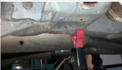
With the front wheels properly blocked; raise the rear end of the vehicle as high as safely possible. Place jack stands on a solid area under the *frame* of the car, not the rear end. Remove the wheels at this time.
