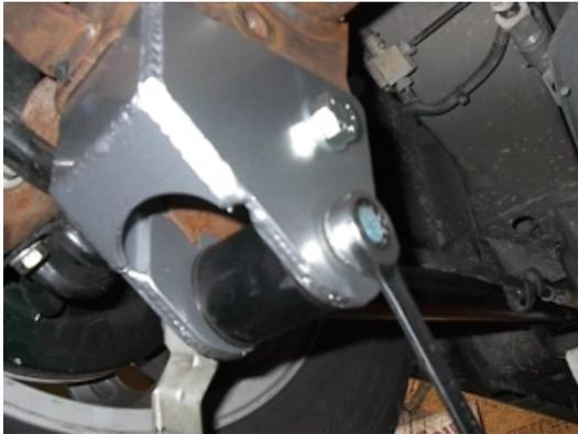
Install the lower control arm into the Anti-Squat Bracket using the provided bolt and washer and the factory flag-nut. It may be necessary to raise or lower the floor jack placed under the pinion to achieve proper alignment. Torque both the control arm and the spacer bolts to 175Nm (129 lb-ft). Remember to tighten front Control Arm bolt if it was loosened.
