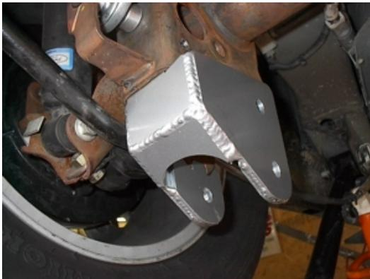
On the Driver's Side of the vehicle, install the Anti-Squat Bracket on the control arm mount of the axle. Inspect the alignment of the Anti-Squat Bracket holes with the factory Control Arm mounting holes. Due to factory variance, it may be necessary to enlarge the hole on the Anti-Squat Bracket for proper alignment. Do not enlarge the factory holes.
