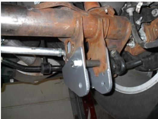
Install the provided 14mm bolt, washers, and lock nut through the provided steel spacer in the factory control arm mounting hole. *Do not fully tighten the bolt at this time.*
