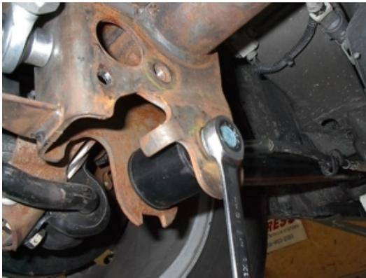
On the Driver's Side of the vehicle, remove the rear (axle side) lower control arm mounting bolt. If you have factory control arms, the front mounting bolt should be loosened but not fully removed. Swing the control arm out of the axle mount. Retain the factory flag-nut for re-use.
