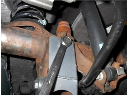
Install the provided 1/2" Flange bolt and lock nut in the slotted hole on the backside of the Anti-Squat Bracket. Torque fastener to 95lb-ft.
