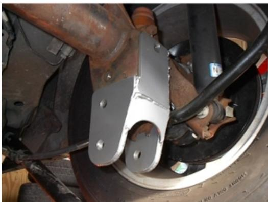
On the Passenger's Side of the vehicle, install the Anti-Squat Bracket on the control arm mount of the axle. Inspect the alignment of the Anti-Squat Bracket holes with the factory Control Arm mounting holes. Due to factory variance, it may be necessary to enlarge the hole on the Anti-Squat Bracket for proper alignment. Do not enlarge the factory holes.
