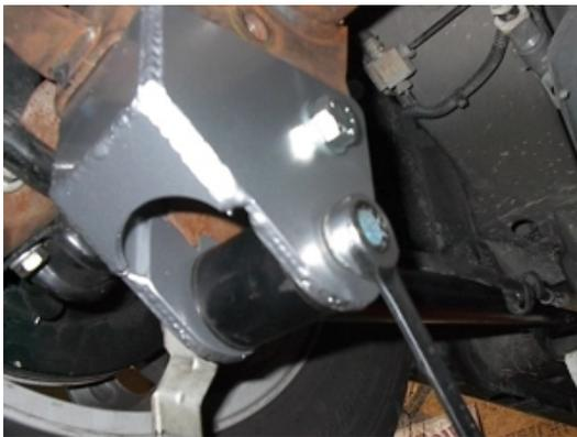
Install the lower control arm into the Anti-Squat Bracket (Driver side shown in photo, Passenger side similar) using the provided bolt and washer and the factory flag-nut. It may be necessary to raise or lower the floor jack placed under the pinion to achieve proper alignment. Torque both the control arm and the spacer bolts to 175Nm (129 lb-ft). Remember to tighten front Control Arm bolt if it was loosened.
