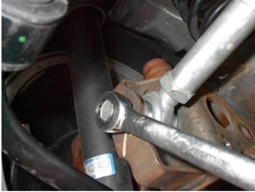
On the Driver's side of the vehicle, loosen the panhard bar bolt. The bolt does not need to be completely removed, but it must be pulled out far enough that it is not protruding into the control arm mounting brackets on the axle. Retain the factory bolt and flag-nut for re-use.
