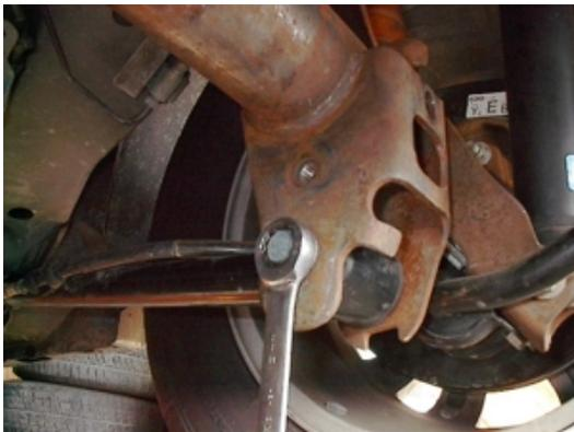
On the Passenger's Side of the vehicle, remove the rear (axle side) lower control arm mounting bolt. If you have factory control arms, the front mounting bolt should be loosened but not fully removed. Swing the control arm out of the axle mount. Retain the factory flag-nut for re-use.
