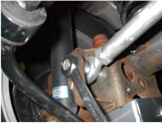
Install the panhard bolt, re-using the factory bolt and flag-nut. Tighten the bolt to 175Nm (129 lb-ft)
