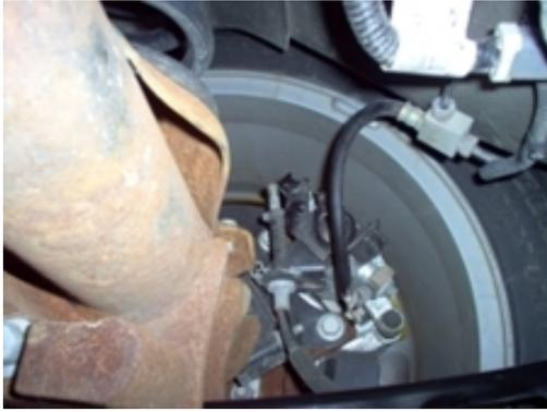
A. Making sure that the parking brake is not applied; disconnect the parking brake cable from the brake caliper by prying the pivot arm down and sliding the cable out of the pivot arm groove.
