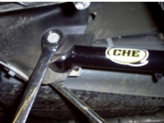
8a. With the parking brake cable retainer facing inboard and the CHE decal right side up, install the control arm in the forward mount. Install the bolt with the nut toward the inside of the vehicle, but do not tighten at this time.
