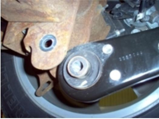
6a. Remove rear mounting bolt allowing the control arms to swing free of the axle mount.
