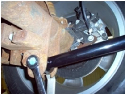
8b. Install the control arm in the axle mount. Install the bolt with the nut toward the outside of the vehicle, but do not tighten at this time.
