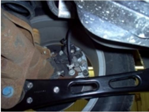
B. Remove the parking brake retainer clip that holds the cable in the caliper and slide the cable out through the control arm.
