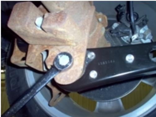
***Working on one side of the vehicle at a time***, loosen, but do not remove, the 2 control arm mounting bolts.
