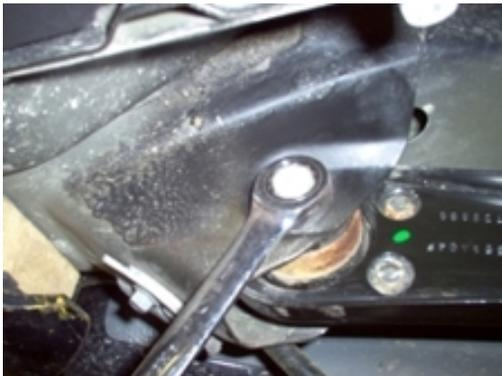
5b. Loosen front mounting bolt
