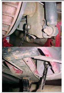
Loosen mounting bolts- Loosen, but do not remove, the 2 control arm mounting nuts.
