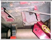
With the spring perch towards the rear of the car and the sway bar mount toward the front, install the control arm in the forward mount. Install the bolt with the nut toward the outside of the vehicle, but do not tighten at this time.
