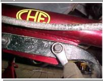
Remove and discard the factory J-clips from the sway bar. Install the new mounting bolts with the nuts toward the outside of the vehicle, remembering to re-install the parking brake/ABS sensor bracket if present. It may be necessary to trim a small amount from the mounting tab of the parking brake bracket to insure a good fit. Torque bolts to 29-37 lb-ft.
