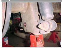
Install rear mounting bolt- Carefully raise the jack until the rear mount is aligned, and install the rear mounting bolt with the nut toward the outside of the vehicle. If the rear end has moved at any time during the installation, it will be necessary to maneuver it back into position.
