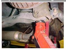
Working on one side of the vehicle at a time, Remove rear mounting bolt- Note: to ease installation, only do one side at a time. Placing the floor jack under the rear of the control arm, carefully raise the jack just until it is supporting the arm and the tension is removed from the bolt-do not apply so much pressure that the rear end is raised.
