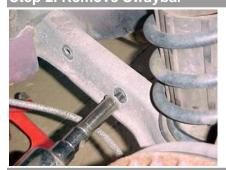
Remove sway bar- Remove the 4 bolts securing the sway bar using a 15mm wrench or socket. If so equipped, remove the ABS Sensor cable from the securing bracket that is mounted to the sway bar bolt. Leave the parking brake bracket on the cable.
