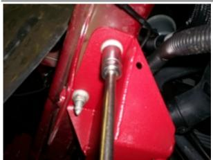
Making sure that all lines are clear and that the radiator is in the proper location, torque the 2 radiator support bracket nuts to 45-50lb-ft. Do this on both sides of the vehicle.
