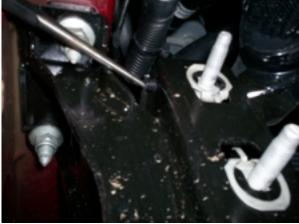
A. Remove the wire harness retainer from the driver's side of the vehicle. Use a punch or other suitable tool to push it through the hole from the backside.
