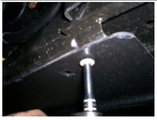
On V8 Models only, remove the 3 screws retaining the front Splash Guard to the Swaybar Crossmember.
