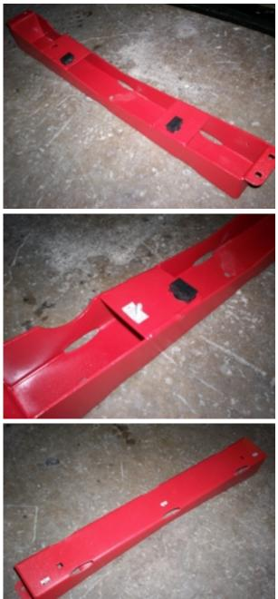
B. Transfer the 2 brake line retainers from the stock crossmember to the new crossmember. Use a suitable removal tool to prevent damage to the retainers.
