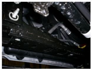
Let the Splash Shield hang from the bumper, it is not necessary to remove the screws retaining the splash shield to the bumper cover.
