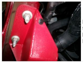
B. Install the electrical line retainer on the Driver's Side of the vehicle into the hole in the rear of the Radiator Brackets.
