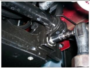
Remove the swaybar from the vehicle by first removing the 2 nuts from the swaybar endlinks attached to the front struts. Remove the 4 nuts retaining the swaybar to the swaybar crossmember and remove the swaybar from the vehicle.
