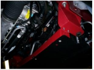
On V8 Models, install the splash shield onto the crossmember using the 3 factory screws.
