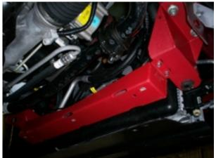
Loosely install the crossmember onto the radiator brackets using the 4 bolts supplied.
