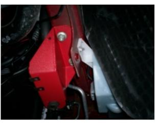
Loosely install the 2 radiator support brackets on the vehicle using the factory Nuts. *Do not tighten the nuts at this time.*
