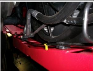
A. Install the brake lines into the retainers on the crossmember. On V8 Models, install the A/C line retainer on the stud using the factory nut.
