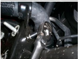
B. On 2007 and later models only, remove the nut retaining the lower coolant hose bracket. Remove the bracket from the vehicle, it will not be re-used.
