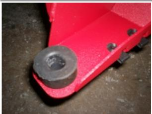
A. Transfer the 2 radiator isolators from the stock crossmember to the 2 new brackets.
