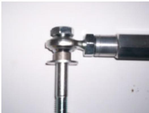
A. Install the rod end spacer and washer so that the washer is toward the bellhousing and the spacer is between the rod end and washer.
