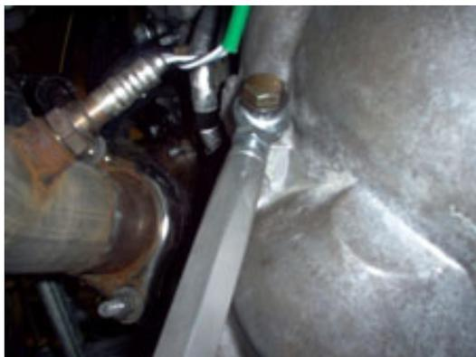
B. Install the limiter link onto the bellhousing using the proper length bolt as specified in chart above. Do not tighten the link jam nut at this time.
