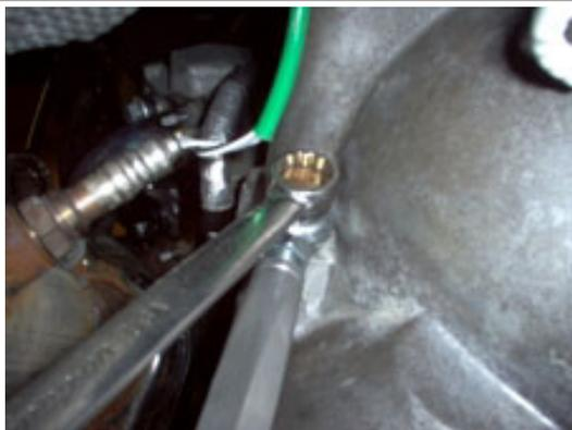
Torque the bellhousing bolt to 33 ft-lbs. Do not tighten the link jam nut at this time.
