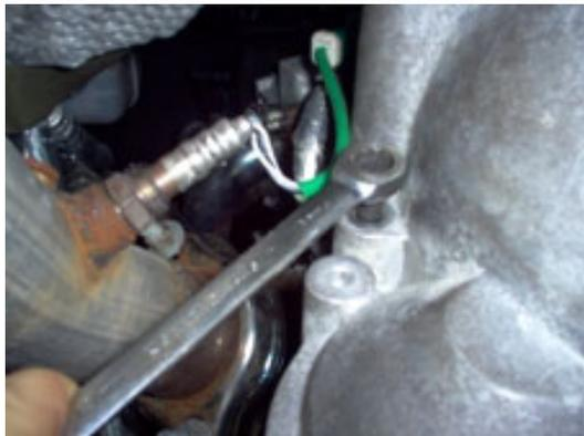
A. Remove the bellhousing bolt located just above the starter housing using a 13mm wrench or socket. This bolt is located on the Driver's side on V6, and on the Passenger side on V8 models.
