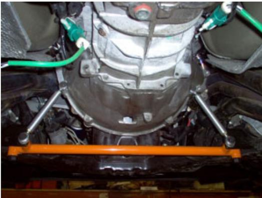
Inspect the installation to insure that there are no clearance issues and that all fasteners are properly tightened. If installation is properly completed, lower the vehicle.
