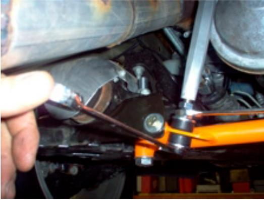
Tighten the bushing jam nut until the bushings are compressed to nearly the diameter of the bushing washers. Do not tighten the bushing assembly so much that the bushing diameter is equal or greater than that of the bushing washers or bushing failure will become possible. Only the jam nut nearest the bushings should be tightened, the second jam nut is used to lock in the Limiter Link after final adjustment.
