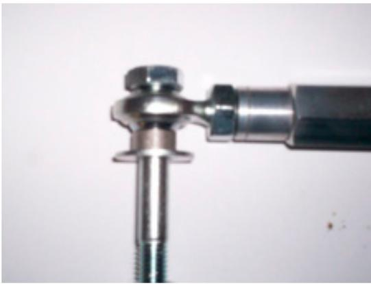
C. Install the rod end spacer and washer so that the washer is toward the bellhousing and the spacer is between the rod end and washer.
