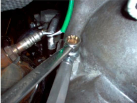
Torque the bellhousing bolt to 33 lb-ft.
