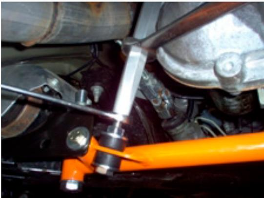
Tighten the Rod End jam nut (remembering that it is a left hand thread) and the bushing end jam nut.
