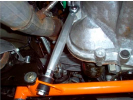
A. Tighten the rod end and bushing assembly (rotate the entire link where needed) into the limiter link until the Limiter length is fully compressed. This step is important to ensure that there is equal thread engagement on both the rod end and the bushing bolt when final adjustment is made. Note that the rod end is a left hand thread.
