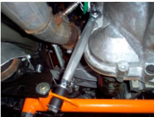
B. Install the bushing assembly through the mounting tab of the K-Member Brace and into the torque link. Remember that there are 2 jam nuts on the Bushing Bolt. ***Do not fully tighten the bushing assembly at this time.***
