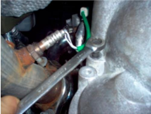
A. Remove the bellhousing bolt located just above the starter housing on V6, or Just below the starter housing on V8 engines, using a 13mm wrench or socket. This bolt is located on the Driver's side on V6, and on the Passenger side on V8 models.
