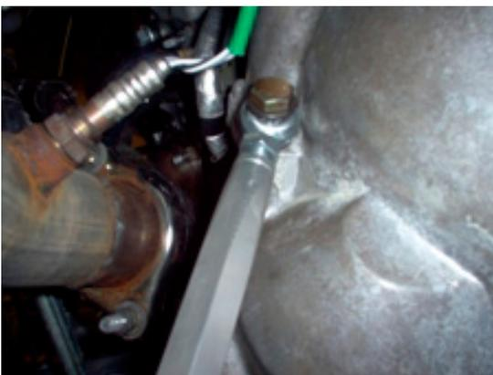
B. Adjust the Limiter length by turning the Limiter Link, ensuring that the rod end or the bushing assembly does not rotate as well. Adjust the length until the bellhousing bolt (with spacer and spacer washer installed as shown in step C) slides into the bolt hole freely.
