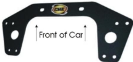
Tip: To ease installation, place large washers over the heat shield studs and install the heat shield nuts to hold the crossbrace in place.
