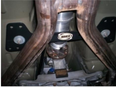
Install the Safety Loop Crossbrace on the vehicle. The large holes in the crossbrace should fit over the raised area surrounding the rearward heat shield stud. Additionally, the 2 notches in the crossbrace (CHE11A only) should be toward the front of the vehicle. On the V6 Manual loop, the crossbrace should be installed as shown in photo at left.
