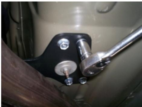
Install the 8 self tapping sheet metal bolts into the holes drilled in step 4. Torque the bolts to 20lb-ft. An impact wrench makes this task much easier, but care must be taken so that the bolts are not over-torqued.
