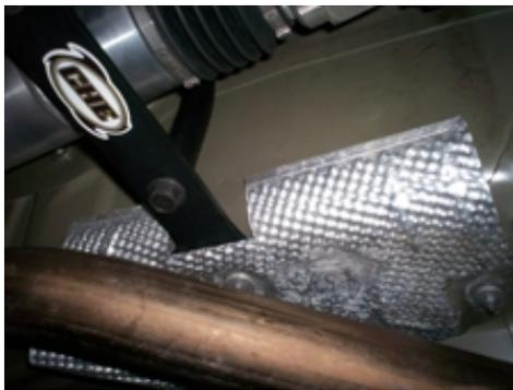
Install the heat shield in the factory location, re-using the factory nuts.
