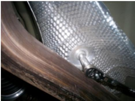
Remove the rear exhaust heat shields (located on either side of the transmission tunnel next to the transmission yoke) from the vehicle by removing the 2 nuts retaining each heat shield. Save the heat shields and nuts for re-use later.
