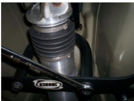
Install the Driveshaft Loop using the provided Flange Bolts. Torque the bolts to 45-50lb-ft.
