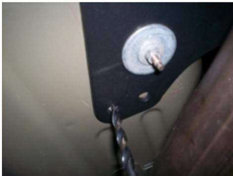
Using a 5/16 drill bit, drill 8 holes for the Crossbrace mounting bolts. It may help keep the holes aligned if a bolt is installed (following the instructions in step 5) before the next hole is drilled.
