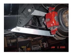
Install the new lower control arm on the vehicle.
