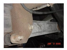
Take caution that the control arm does not swing down causing vehicle damage or bodily injury when the bolts are loosened.
