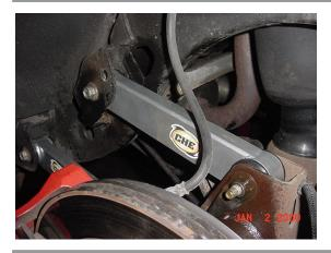
A. Lubricate the bushing faces and mounting points of the upper control arm following instructions in step 5.
