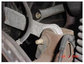
Take caution that the control arm does not swing down or that the flag nut does not rotate causing vehicle damage or bodily injury when the bolts are loosened.
