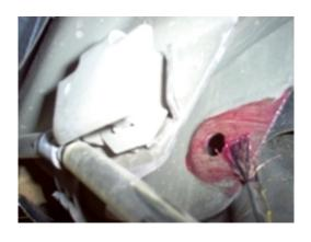
Fully inspect all mounting points and remove any debris. Apply a light coating of the supplied synthetic grease to all surfaces that will be in contact with the bushings. At this time, also coat the outside of the bushings themselves with the same supplied grease
