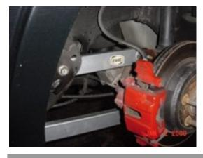
Install the lower and upper control arms on the second side of the vehicle following steps 4 through 10.
