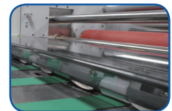
AUTOMATIC FEEDING GAP CONTROL DEVICE
