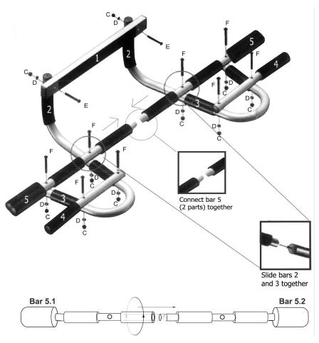
Connect Bar 5.1 and Bar 5.2 together by rotating clockwise.
