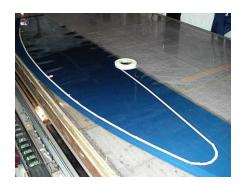
Draw the shape of the window required onto the window material.
