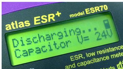
It can measure and compensate for the effects of measuring ESR in-circuit too, it also knows that you don't want to be hassled with capacitor polarity, just connect any way round.
