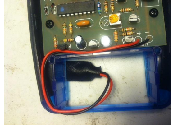
Battery Lead Dress
