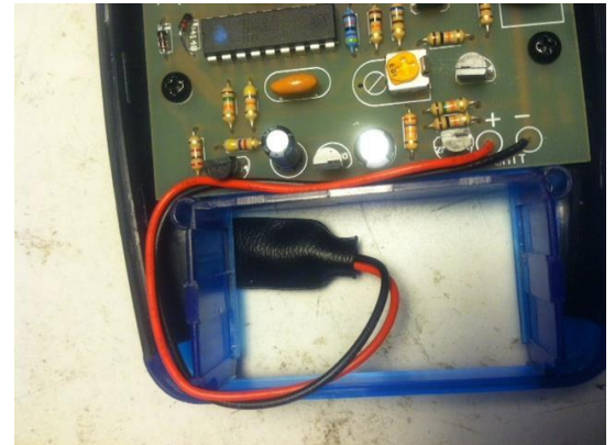
Battery Lead Dress
