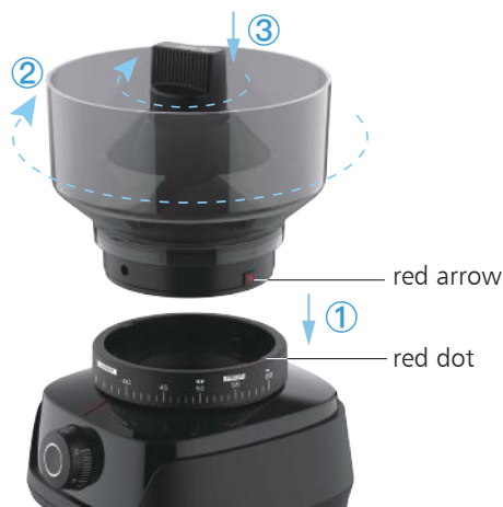
Fig.2 Assemble bean hopper
