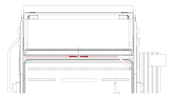
6. Make sure that you have 7 screws remaining for this step. Drill a hole(Ø3.2mm) 1 cm from each edge of the velcro. Measure the distance between these 2 holes and then divide the distance for the remaining 5 screws. This measurement should be approximately ~24,5cm. (Part used: F)
