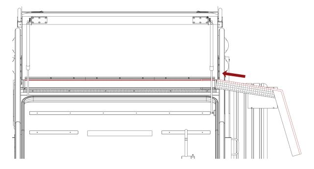
**8.** Attached the Loop Velcro to the Hook. Ensure it is properly attached.
