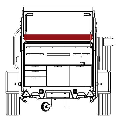
**2.** Drill(Ø3.2mm) the rivets in the top velcro. If the lower part of the velcro is intact it can be reused, otherwise drill out the rivets here as well. **Do not drill deeper than 20mm.**
