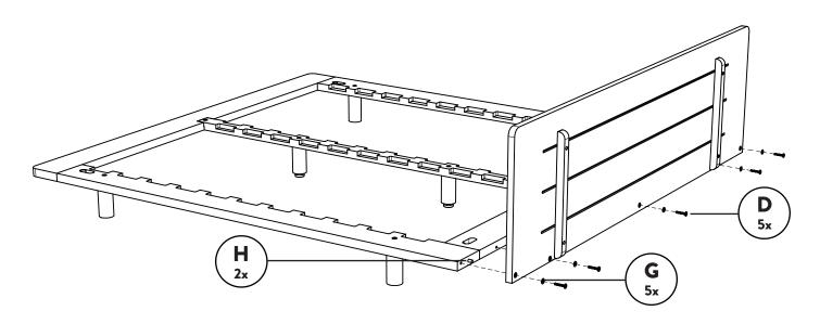
Install 2x dowels (H) to the bed frame, then install the headboard (9) using 5x bolts (D) and 5x washers (G).
