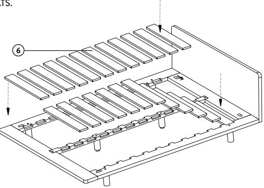
Fit the slats (6) by simply placing them onto the slots on the bed frame.
