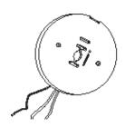
50W electronic transformer included in monopoint. Allows for one low voltage track NTL-2200 series track head. Mounts permanently to outlet box.
