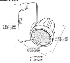
Width: 4-1/2" (12W) / 6-1/2" (23W) Lenath: 3-5/8" (12W) / 4-1/4" (23W) 2-5/8" (12W) / 3-5/8" (23W) Diameter: Max. Extension: 7-1/2" (12W) / 8-1/2" (23W)
