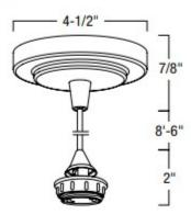
Canopy Diameter: 4-1/2" Canopy Depth: 7/8" 8'-6" Cable Length: Socket Length:
