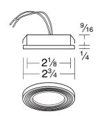
Fixture Diameter 2-3/4" Housing Diameter 2-1/8" Fixture Height 1/4" Housing Height 9/16"
