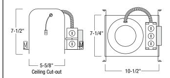
Cut-out: 5-5/8" ID: 5" OD: 5-1/2" Housing Length: 10-1/2" Housing Width: 7-1/4" Housing Height: 7-1/2"
