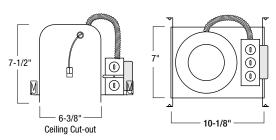
Cut-out: 6-3/8" ID: 6" Housing Length: 10-1/8" Housing Width: 7" Housing Height: 7-1/2"
