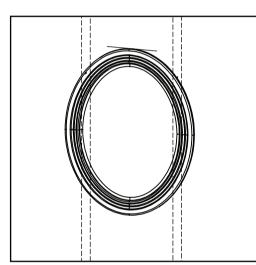
Mark the top of the mirror on the wall. Ensure Mirror is centered between studs, see Caution Above
