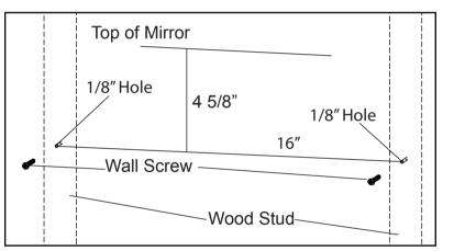
Mark the location to install the screws. Each screw should be centered on a wood stud, see caution above. The holes should be 4 5/8" (118mm) below the mark for the top. Pre-drill each hole using a 1/8" drill bit (not included) Install the screws so that the hanger will fit over the head of the screw (approximately 3/16" (4mm) from wall).
