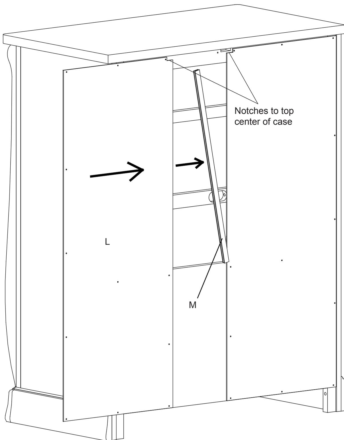
Insert The Panel Joint (Part M) to the Back Panel, then insert the (1) Back Panel (Part L) into the slot of Panel Joint.
