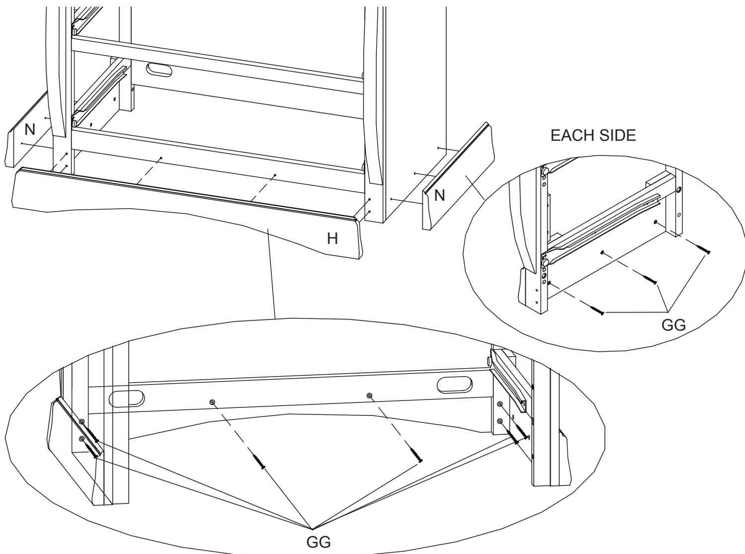
Attach the Bottom Front Molding (Part H) to the front of the case using (8) 30mm Screws (Part GG), ensure the screws go into the predrilled holes in the molding. Tighten with a Phillips screwdriver. Next attach the (2) Bottom Side Moldings (Part N) to the case using (3) 30mm screws (Part GG) for each, ensure the screws go into the predrilled holes in the molding.
