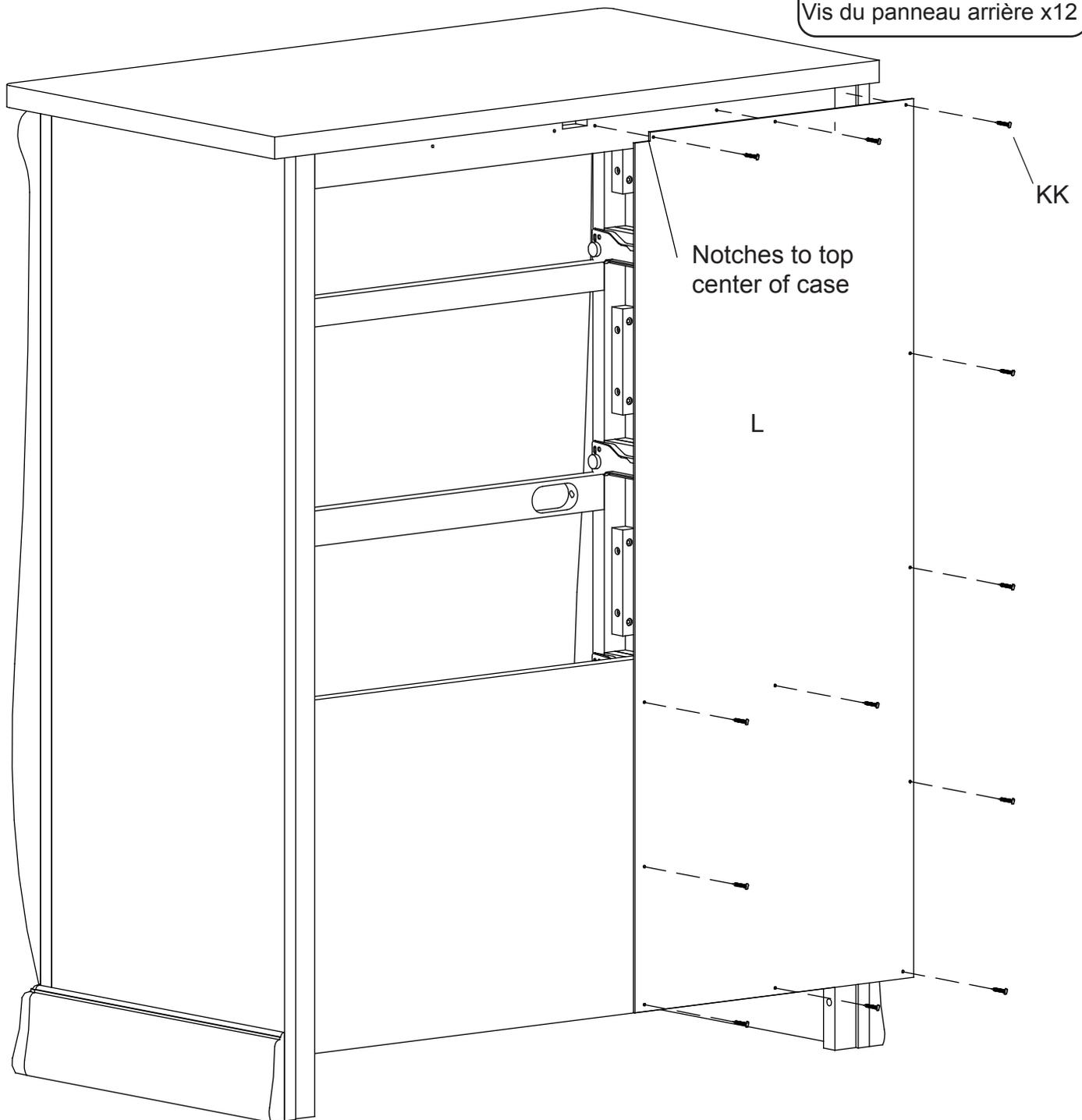
Attach ( 1) Back Panel (Part L) using (12) Back Panel Screws (Part KK). Tighten with a Phillips Screwdriver.
