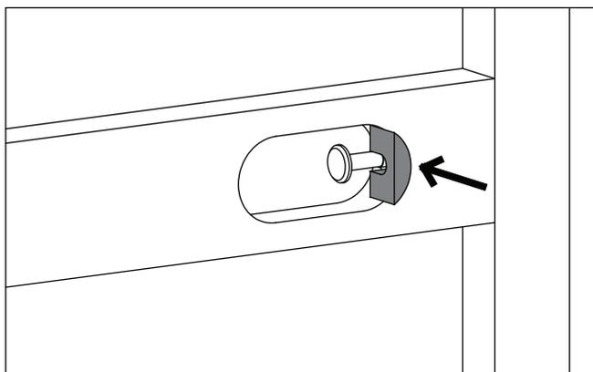
Slide the Plastic Crescent Washer over the exposed bolt, behind the head of the bolt. Tighten the bolt with the M5 Allen Wrench provided.
