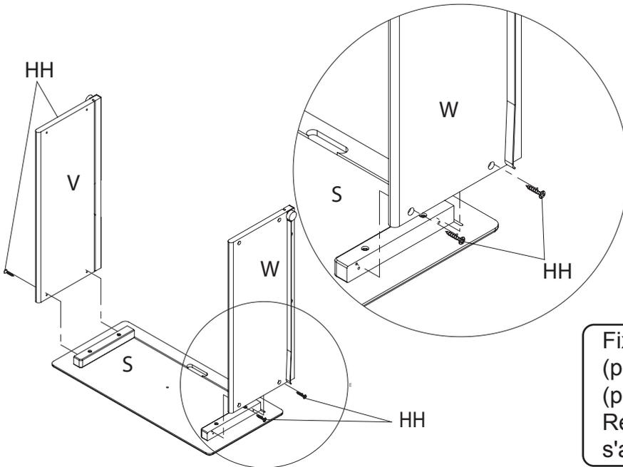
Attach the Right and Left Drawer Sides (Parts V And W) to the Drawer Front (Part S) with (4) 25mm Screws (Part HH) Note: Grooves In Bottom Must Align. Tighten With Phillips Screwdriver
