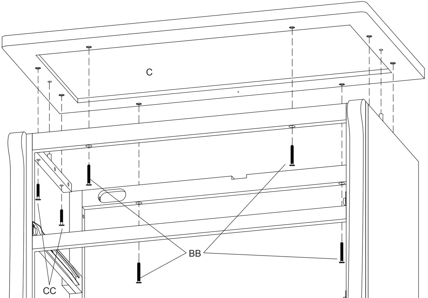
Attach the Top Panel (Part C) to the case. Ensure (2) Dowels from the side are aligned properly before installing any bolts. Install (4) 45mm bolts (Part BB) through the Top Front and Back Rails, then install (4) 35mm Bolts (Part CC) through the sides. Tighten all bolts with the M4 Allen Wrench.
