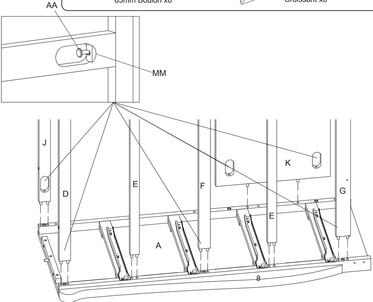
Attach Top Front Rail (Part D), Middle Front Rail (Part F), Bottom Front Rail (Part G), (2) Drawer Rails (Part E), Top Back Rail (Part J) and Bottom Back Rail (Part K) to the Left Side (Part A). Carefully align all of the Dowels with the holes in the Left Side (Part A). Attach the rails to the Left Side using (6) 65mm Bolts (Part AA) and (6) Crescent Washers (Part MM) following the direction on page 5. Tighten all bolts with Allen Wrench.
