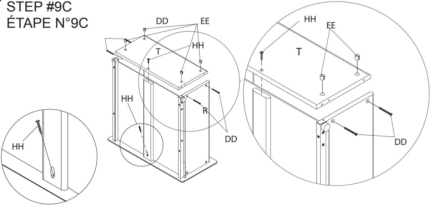
Install the Drawer Support (Part R) and Drawer Back (Part T), using (2) 25mm Screw (Part HH), (4) 40mm Screws (Part DD) and (4) Plastic Barrel Nuts (Part EE). Note: Grooves In Bottom Must Align. Tighten With Phillips Screwdriver
