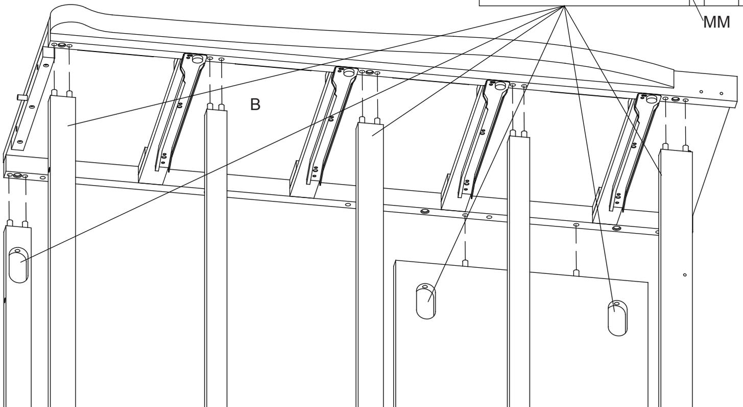
Repeat Step 2 using the Right Side (Part B). Refer to Page 5 to install the 65mm Bolt and Plastic Crescent Washer.
