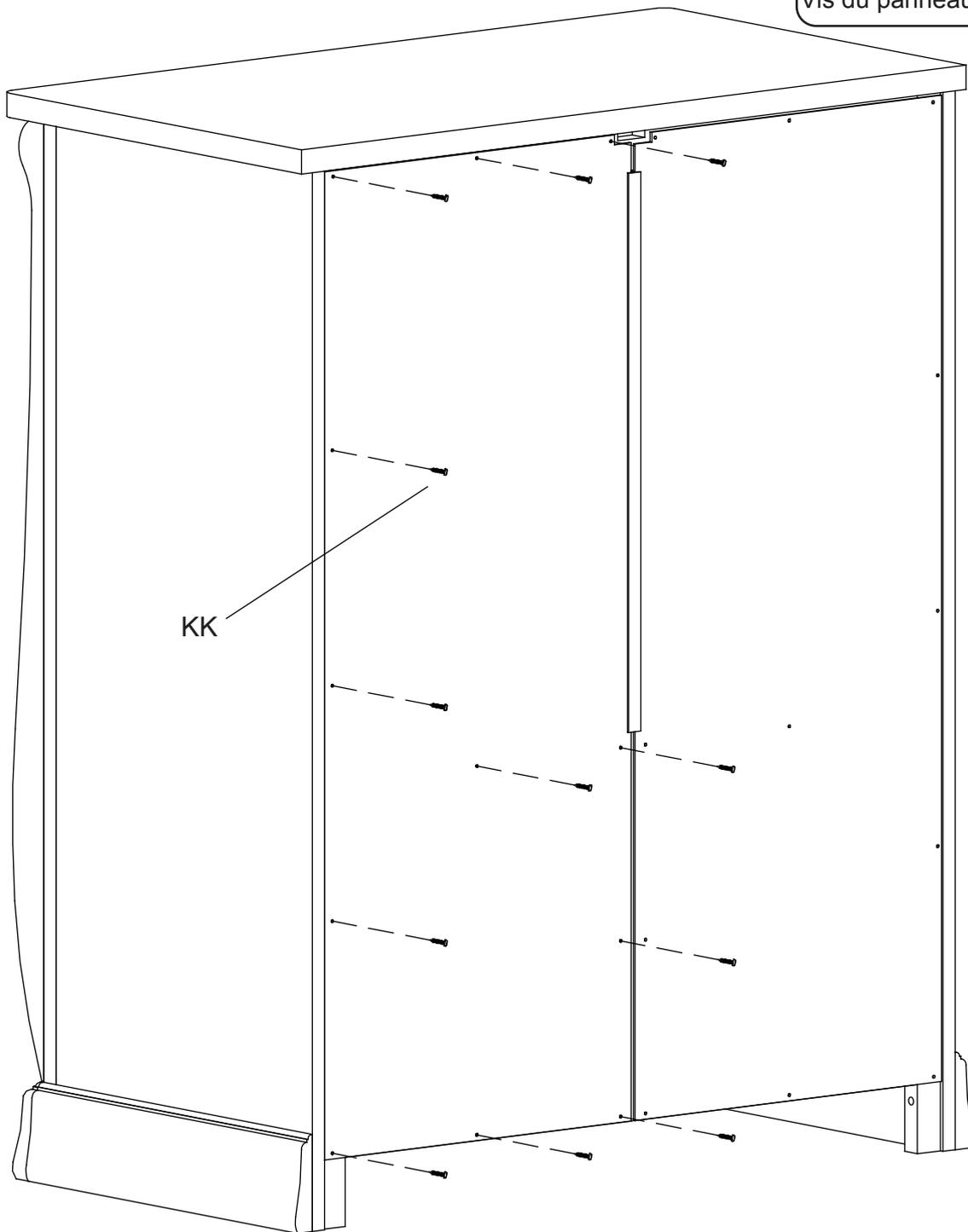
Attach ( 1) Back Panel (Part L) using (12) Back Panel Screws (Part KK). Tighten with a Phillips Screwdriver.
