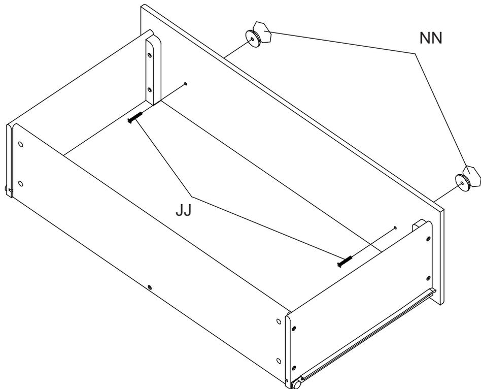
Attach (2) Knob (Part NN) with (2) Knob Screw (Part JJ) Tighten With The Phillips Screwdriver.
