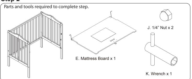
Attach (1) Mattress Board (Part E) to the assembly from step 1 using (2) 1/4" Nuts (Part J), Tighten with the Wrench (Part K).
