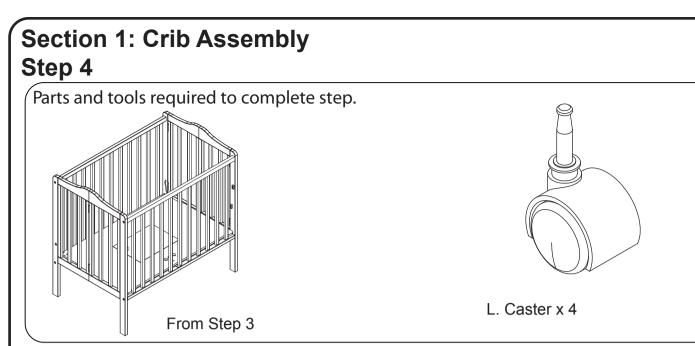
Insert the (4) Casters (Part L) into the Legs of the Crib. Attach each Caster by pressing firmly until it "Snaps" into place. Do not insert the Casters by pounding the ends of the Crib on the floor, this will damage the unit.
