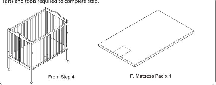
Place the Mattress Pad (Part F) onto the Mattress Board (Part E) as shown.
