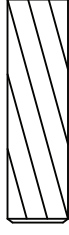
KK. M8x30mm Wood Dowel x2 Cheville en Bois M8x30mm Pasador de Madera M8x30mm
