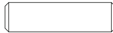
KK. Φ8x30mm Wood Dowel x46 Cheville en bois Φ8x30mm Pasador de madera Φ8x30mm
