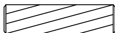
KK. M8x30mm Wood Dowel x2 Cheville en Bois M8x30mm Pasador de Madera M8x30mm
