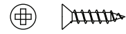
M. Hingle Screw - Flat Head 12mm x 8 Tornillo de la bisagra x 8
