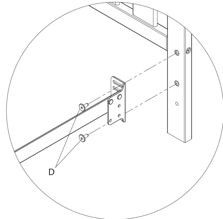
If there are inserts use 2 (part D) 16mm bolts per post tighten with allen wrench.
