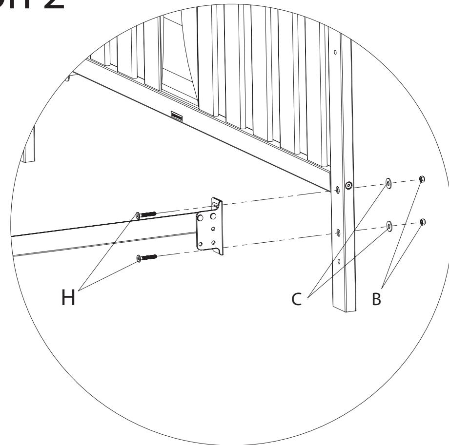
If through holes use 2 nuts (part B), 2 washers (part C) and 2 bolts (part H)
