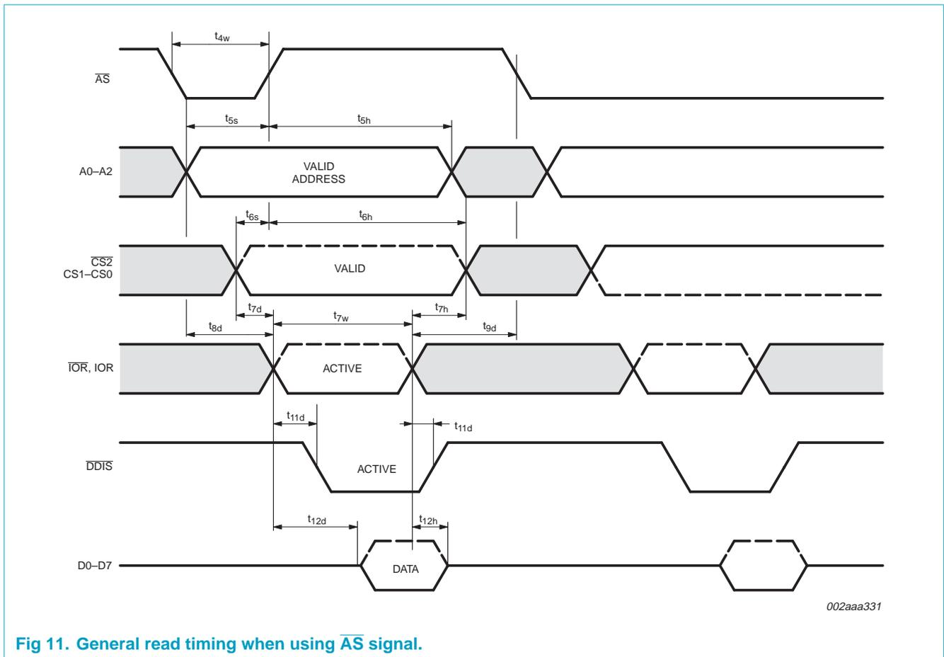
Fig 11. General read timing when using  $\overline{\text{AS}}$  signal.
