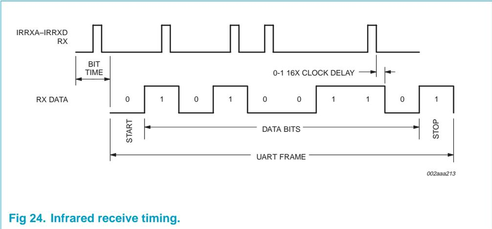
Fig 24. Infrared receive timing.
