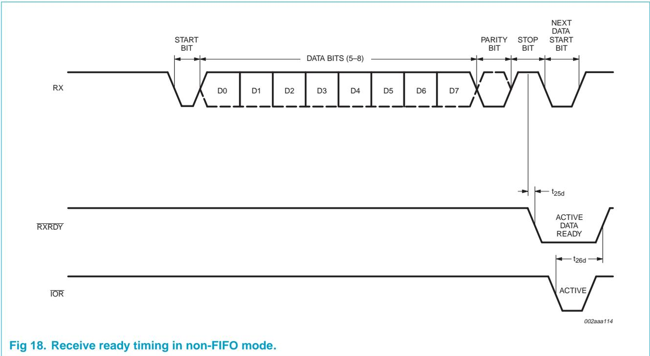
Fig 18. Receive ready timing in non-FIFO mode.
