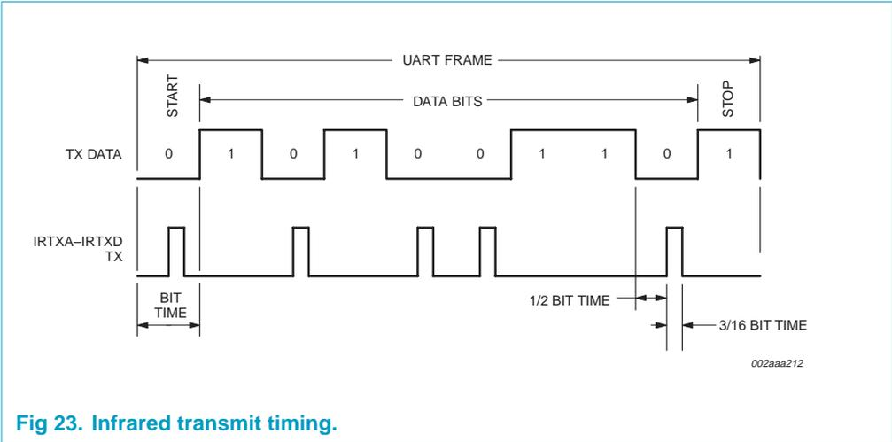
Fig 23. Infrared transmit timing.
