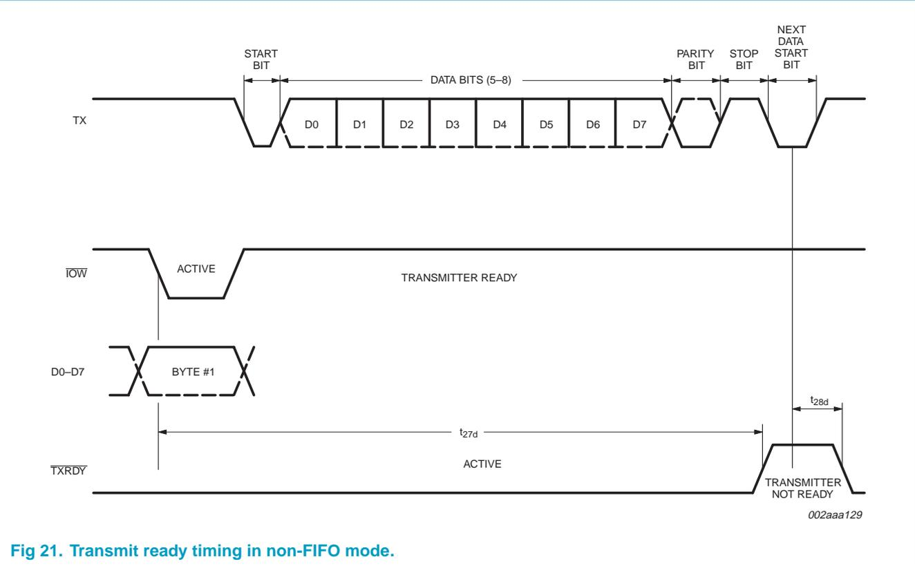
Fig 21. Transmit ready timing in non-FIFO mode.
