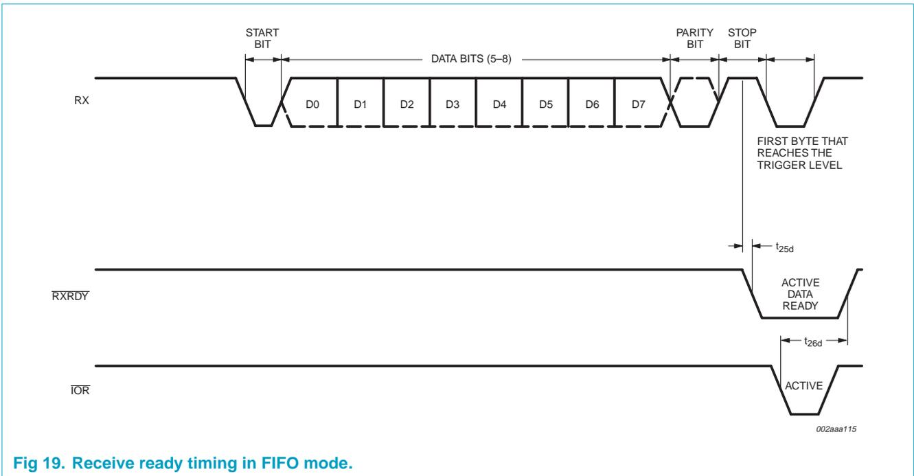
Fig 19. Receive ready timing in FIFO mode.
