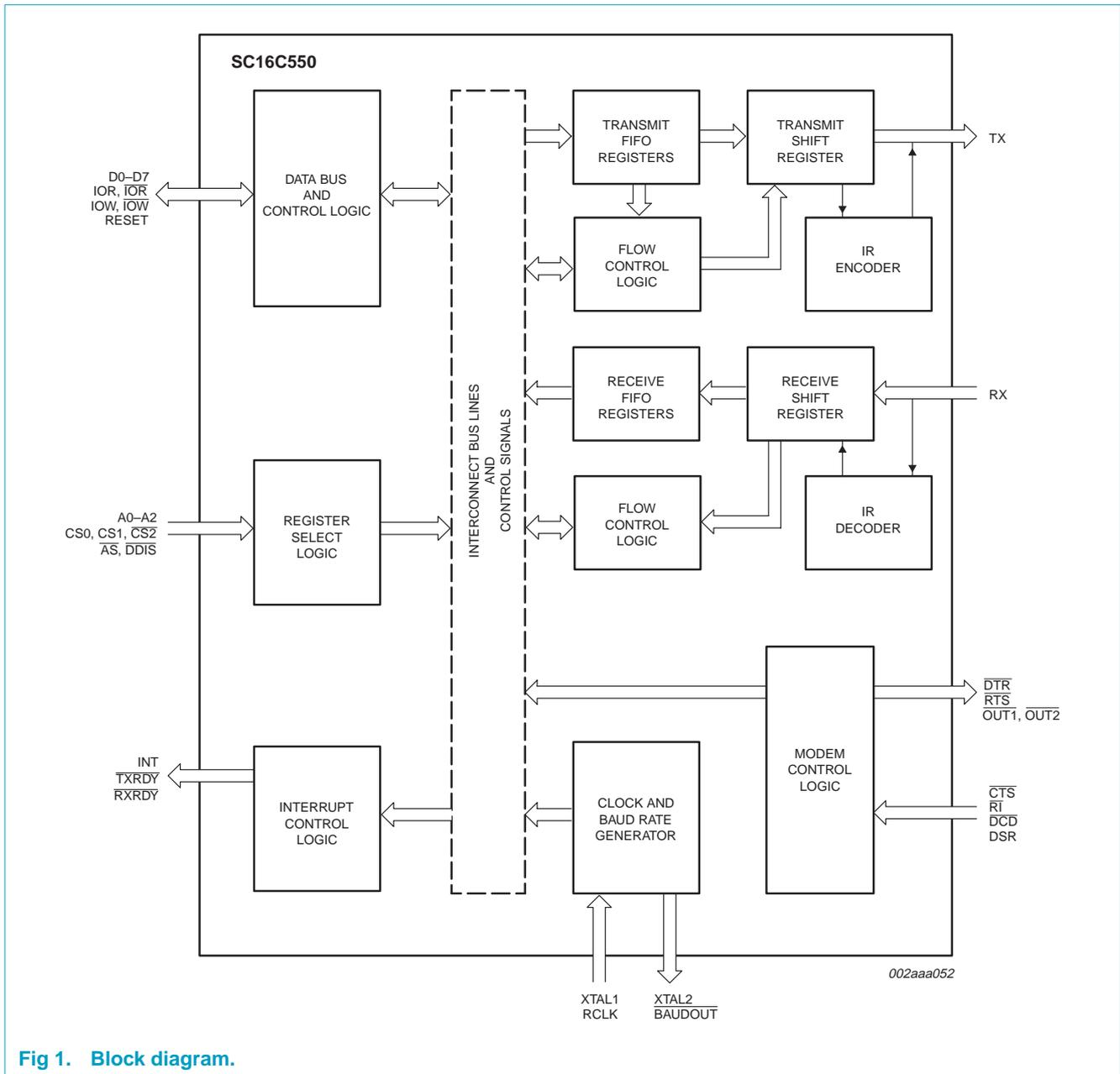
Fig 1. Block diagram.
