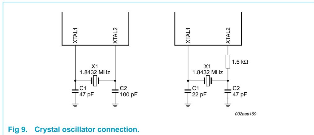
**Fig 9. Crystal oscillator connection.**
