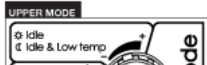
Turn knob between <<->> and <<+>> signs in UPPER section to set idle speed.
