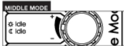
Turn knob between <<->> and <<+>> signs in MIDDLE section to set idle speed.
