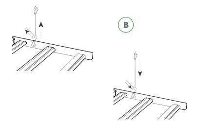
Lift the LED and attach the carabiners to pre-installed hooks from ceiling or mounting beam. The Ratchets should be installed closest to the LED (and not the ceiling).
