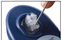
remove reagents which coat the CELL wall.
