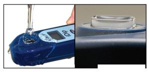
**CAP CELL AND ZERO METER** Place the Cell Cover onto the CELL and eXact iDip® 570 photometer display rea
