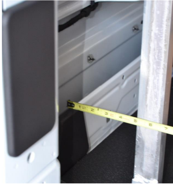
Rear Single Channel Unistrut 5" Off Side Wall
