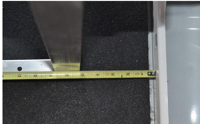
Front Single Channel Unistrut 5" Off Side Wall
