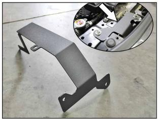
Locate passenger-side Upper Mounting Bracket. Carefully insert the bracket into the cavity behind the grille. Rest the bottom of the bracket on the bumper beam and ensure the mounting holes align with the bolts on top.
