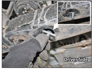
Insert the 3/8"-16 x1.5" Bolt Plate (Offset) into the larger driver-side hole like shown. Slide (1) card square onto the threads until it bottoms out against the chassis. This will prevent the bolt plate from moving around during assembly. Note: This bolt plate has the threaded stud closer to the center of the plate.
