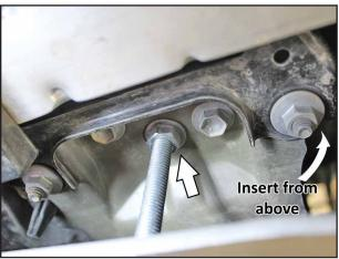
Insert (1) 3/8"-16 x4.25" Hex Bolt and Flat Washer into each hole (bolt threads facing down). Fasten them in place with a 3/8" Flat Washer, Lock Washer and Hex Nut. Center the bolt in the hole & tighten nut down. Repeat on passenger side.
