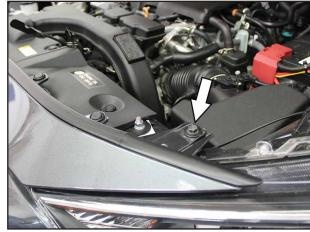
Remove this 10mm-head bolt on the front bumper, on both sides (driver and passenger area). This will help in removing the air diverter panel.
