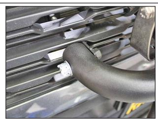
Install the light bar by inserting (1) 3/8"-16 x2" Hex Bolt, 3/8" Lock Washer, and 3/8" Flat Washer through each hole on the upper tube of the Light Bar and into the threaded holes on the Grille Brackets.
