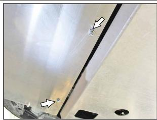
Locate the Skid Plate and align the rear holes with the bolt plates. Fasten the rear bolt plates with (1) 3/8" Flat Washer, Lock Washer, and Hex Nut on each bolt. Do not tighten.
