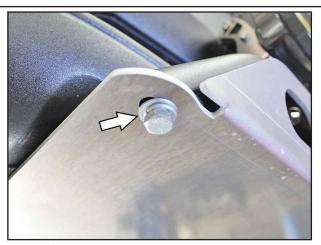
Locate the front holes and align with the bottom mount holes on the Light Bar. Fasten (1) 3/8"-16 x1" Hex Bolt, Lock Washer, and Flat Washer into each hole. Tighten down bolt.
