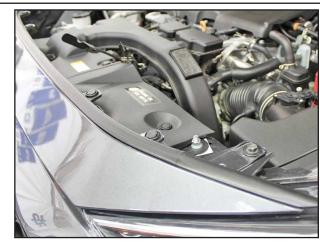
Reinstall air diverter panel in the engine bay.
