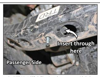
Insert the 3/8"-16 x1.5" Bolt Plate into the passenger side hole.
