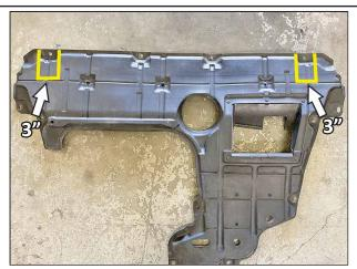
Trim the splash guard in the areas shown and reinstall. Each rectangular cut is 3" wide x 5" long and up to the indentation shown in the splash guard. Note: Adventure models have a smaller splash guard but the location and size of the cutouts still applies.
