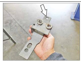
Place a 1/2" Washer on the rear-most hole on the lower mounting bracket so that it is sandwiched between the chassis and the bracket when it is installed.
