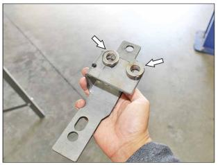
Place cylindrical spacers on top of the mounting holes on the driver side Lower Mounting Bracket. Repeat on the passenger side bracket.
