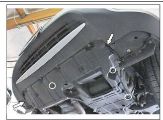
Remove the engine splash guard by unfastening the plastic fasteners underneath.
