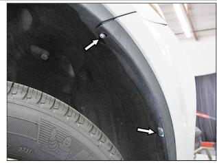
Unfasten the (2) screws in the fender well area on each side of the vehicle.
