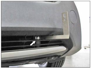
Reinstall the front bumper, but do not reinstall the bottom fasteners yet. Attach the Grille Brackets to the Upper Mount Bracket with (1) 1/4"-20 x3/4" Hex Bolt, (1) 1/4" Lock Washer, and (1) 1/4" Flat Washer into each hole. (Driver side shown) Repeat on passenger side.
