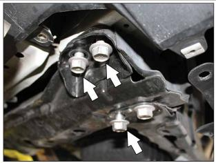
Locate the (3) chassis bolts shown above on the driver side. Remove these bolts.
