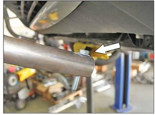
Install (1) 3/8"-16 x2.5" Hex Bolt and (1) 3/8" Flat washer on each end of the light bar at the lower mounting holes.
