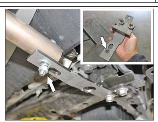
Insert the 3/8" Bolt on the Light Bar into the front hole on the lower mount bracket. Fasten the 3/8" Bolt with (1) 3/8" Flat Washer, (1) 3/8" Lock Washer, and (1) 3/8"-16 Hex Nut on each end of the Light Bar. Do not tighten yet.
