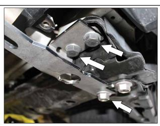
Attach the Bracket to the chassis using (1) M12 x110mm flange bolt at the rear and (2) M12 x45mm flange bolts through the middle of the bracket and the cylindrical spacers. Repeat process on the passenger side. Tighten down all hardware.
