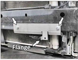
Install the driver side Upper Mount Bracket by lining up the holes with the rivet nuts and fastening them with (1) 1/4"-20 x3/4" Hex Bolt, (1) 1/4" Lock Washer, and (1) 1/4" Flat Washer into each hole. Repeat on the passenger side.
