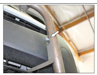
Attach the light bar to the upper holes on the Grille Brackets with a 5/16"-18 x1" Hex Bolt, 5/16" Lock Washer, and 5/16" Flat Washer in each hole. Keep the bolt loose for now to allow the bar to pivot around in next steps.
