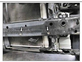
Locate the (2) holes shown above on the bumper beam (driver side shown). Install (1) 1/4"-20 Rivet Nut into each hole using a Rivet Nut tool. Locate the mirror-opposite holes on the passenger side and repeat.
