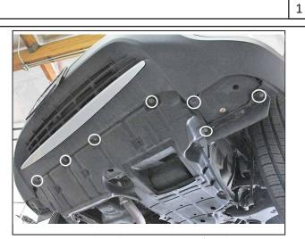
Remove the (4) 10mm-head screws under the front bumper and the (2) 10mm-head screws under the fog light area on both sides of the vehicle. The bumper should now be free from the vehicle (unplug the fog lights from the wire harness if vehicle is equipped).
