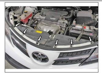
Remove front bumper. Start by removing the fasteners at the top of the bumper under the hood.
